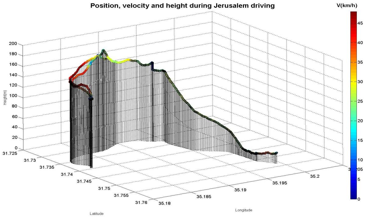
Figure 10: Vehicle's location (coordinates and map), velocity and relative height while driving in Jerusalem.
